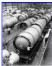
*Figure 43: TITAN III Core Vehicle Fuel and Oxidizer Tanks*
